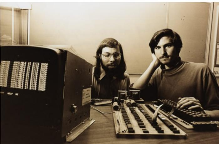
microprocessor, MOS's Technology 502. This was his new goal in life. While keeping his job at HP, he worked very hard at this computer board, and came up with an impressive result; a powerful computer (for the time) which worked with a keyboard and screen, not one that flashed lights — and all with amazingly few chips.
